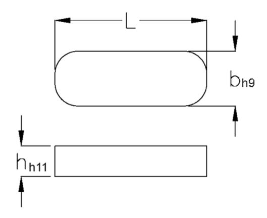
$\begin{array}{ll} b & = 14 \\ h & = 9 \\ L & = 220.0 \\ Tolerance \ b = 0.043 \\ Tolerance \ h = 0.090 \\ Tolerance \ L = -0.5 \end{array}$
